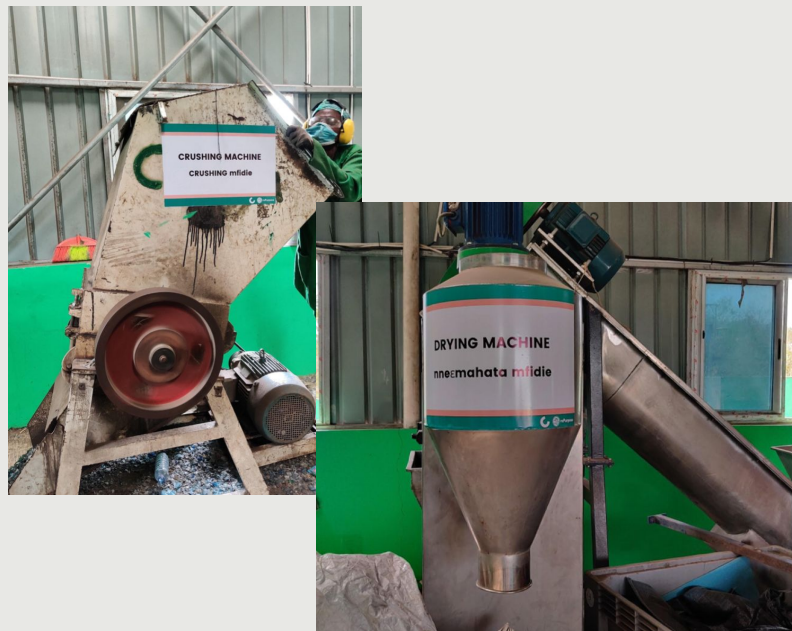
Crushing, Washing & Drying Of Flakes
